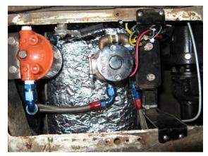
After installing the Reflecta Shield I then installed the shield assembly to the top of the muffler with the three included band clamps. In the photos you can see the Dan Walters Torque Arm assembly. The heat shield assembly has proven extremely effective and it has reduced the muffler radiated temperature by roughly 87 degrees from muffler temp
