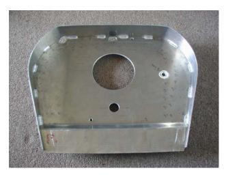
With all of the pieces made and test fitted take everything out to a specialist and get them welded. About \$80-\$100 is a reasonable amount for quality work. I had Rod at **Twisted Metal Motor Cycle Fabrication** in Lake Forest, CA weld mine and he did an absolutely SUPERB job. Be sure to have the outside continuously welded with several stitches on the inside to minimize cracking due to flexing of the part. Having a pro do it makes all the difference in the appearance of the welds.
