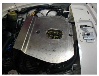
template to allow for the distributor cap to clear the base plate with a margin of safety. (On the template I have available for others I traced the actual base bend side profile for reference.)
