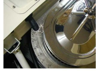
deform my chrome restored lid, not a desirable solution for me. Having the base orient or register on the fuel bowl adjustment nuts solved this 'walking' issue for me.
